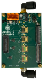
(a) First SMB prototype (SMB1) with four MuTRiG 1 chips and connectors at the right of the picture to connect to a SiPM array
