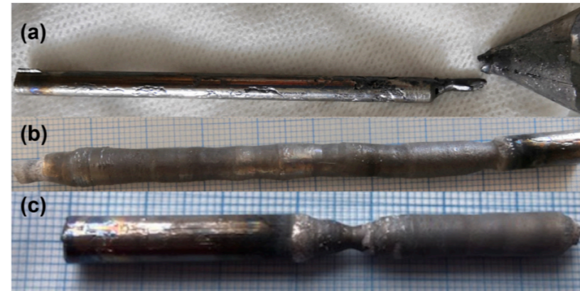
FIG. 3. Photos of (a) the cast CeAlGe rod, and the floating-zone-grown crystals of (b) CeAlGe and (c) PrAlGe.
