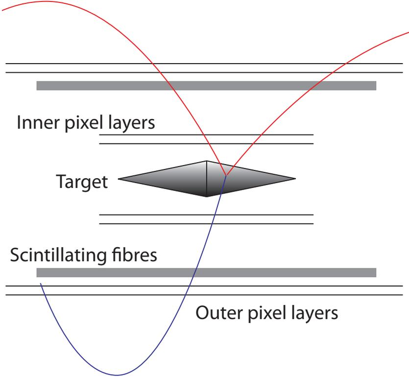
Make a compact detector, long enough to catch the particles after half a turn.
