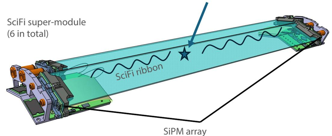
Particles produce photons which propagate towards the ends
