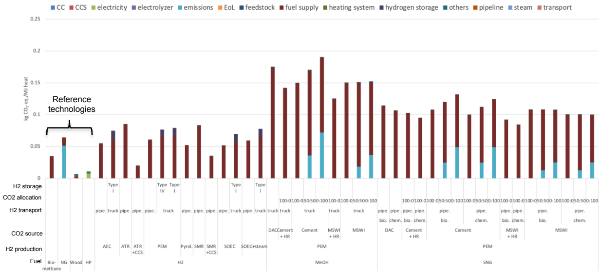
Figure 69 Life-cycle Global Warming Potential impacts per MJ of heat supplied for all boiler-based options, in addition to reference options. All cases where the hydrogen is supplied via a PEM electrolyzer (“PEM”) use Swiss grid electricity. “NG” = natural gas-fed boiler. “Wood” = wood-fired boiler. “HP” = air-water heat pump powered with Swiss grid electricity. “pipe.” = hydrogen transport by pipeline. “truck” = hydrogen transport by truck. “PEM” = Proton Exchange Membrane fuel cell or electrolyzer. “ATR” = Auto-Thermal Reforming of natural gas. “SMR” = Steam Methane Reforming of natural gas. “bio.” = biological methanation. “chem.” = electrochemical methanation. “DAC” = atmospheric carbon dioxide captured by Direct Air Capture. “Cement” = carbon dioxide, captured at cement plant. “MSWI” = carbon dioxide, captured at municipal solid waste incineration plant. “100:0” = carbon dioxide emissions allocated to emitter. “50:50” = carbon dioxide emissions allocated equally between emitter and fuel producer. “0:100” = carbon dioxide emissions allocated entirely to fuel producer. “CC” = carbon dioxide capture/sourcing. “CCS” = carbon dioxide capture and storage. “EoL” = End-of-Life.
